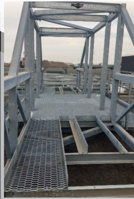
Custom Walk Around for Motor and Drive
